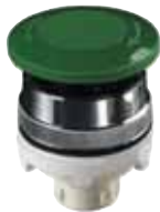
Automatic Push/Turn Mushroom. Manual push "In". Latches "In". Turn clockwise to unlatch. Spring return.
