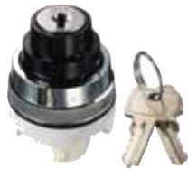
Key Twist 90° Maintained. (PL- T3K-B) Turn key clockwise to latch "In". Turn key counterclockwise to release. Key with-drawable in both positions. Black only.
